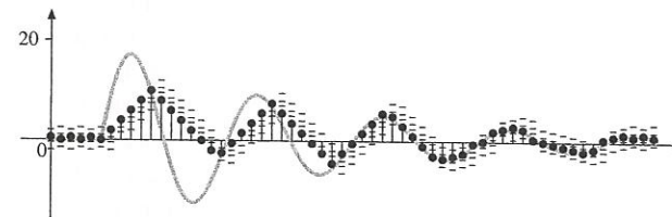
Figure 8.7 Action of a DPCM encoder and decoder on an example signal.
